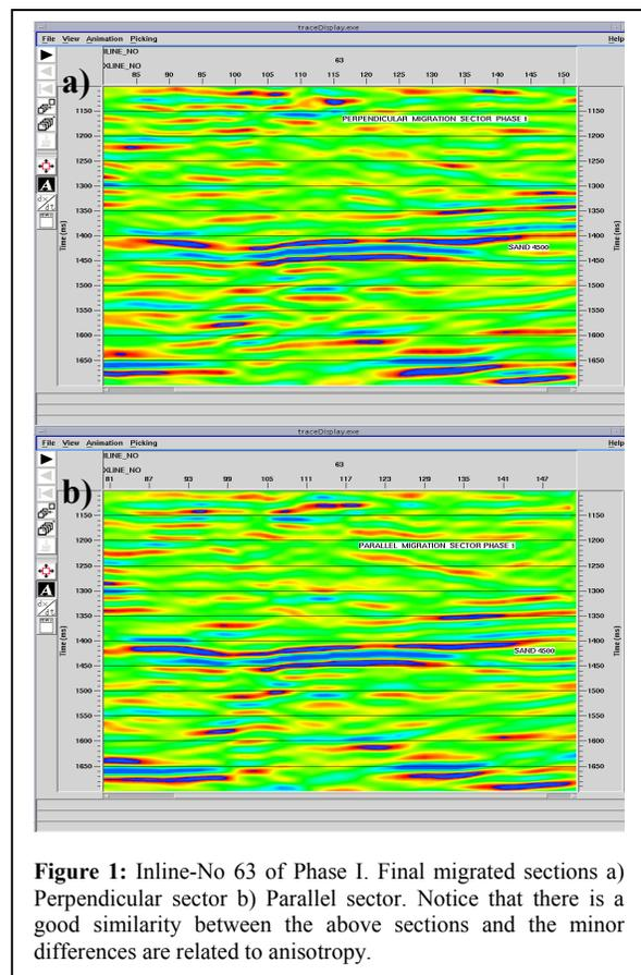
Figure 1: Inline-No 63 of Phase I. Final migrated sections a) Perpendicular sector b) Parallel sector. Notice that there is a good similarity between the above sections and the minor differences are related to anisotropy.
