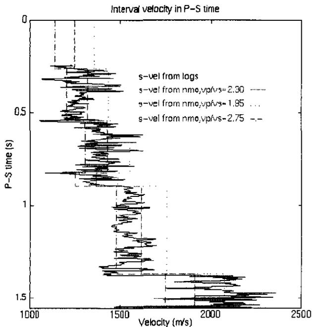
**Fig. 6.** Comparison of Dix estimates from the velocity analysis of Figure 5 to the S-wave well log. The effect of changing  $\gamma$  (from 1.09 to 2.75) is shown in the plot.
