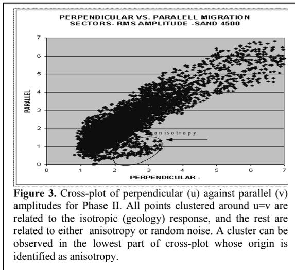
**Figure 3.** Cross-plot of perpendicular (u) against parallel (v) amplitudes for Phase II. All points clustered around  $u=v$  are related to the isotropic (geology) response, and the rest are related to either anisotropy or random noise. A cluster can be observed in the lowest part of cross-plot whose origin is identified as anisotropy.
