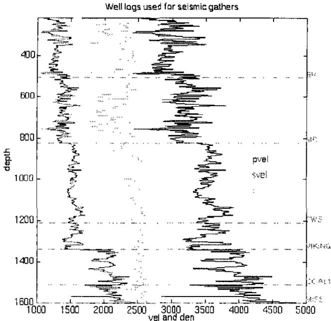
Fig. 2. Logs used to generate the P-S gather of Figure 4. The S-wave velocity (left) was derived from the P-wave velocity (right) using a depth varying  $\gamma$  (Figure 3).
