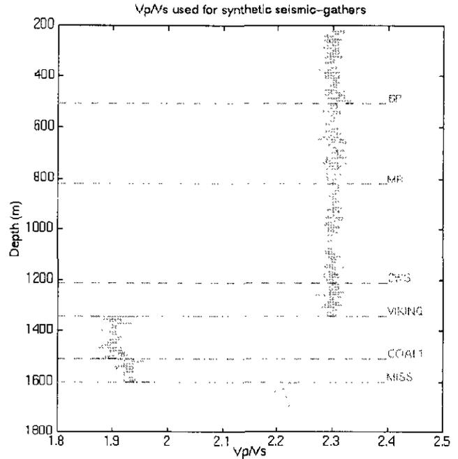
Fig. 3. Depth varying  $\gamma$  ( $V_p/V_s$ ) used in estimation of S-wave velocity.
