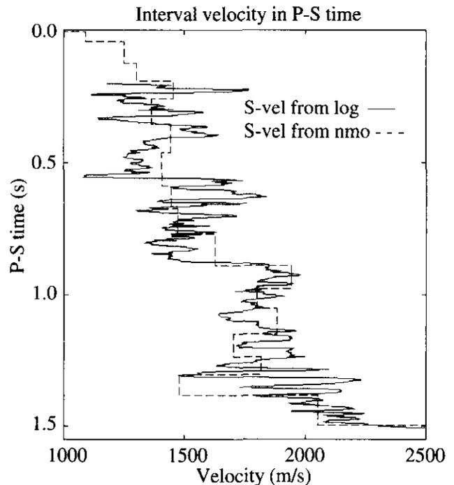
**Fig. 7.** a) Stacking velocity from the Blackfoot 2D - 3C. Comparison of the Dix estimate to an S-wave log from the area. The  $\gamma$  estimate is high ( $\gamma = 3.25$ ) due to picking the stacking velocities (a) based on large-offset NMO semblance.
